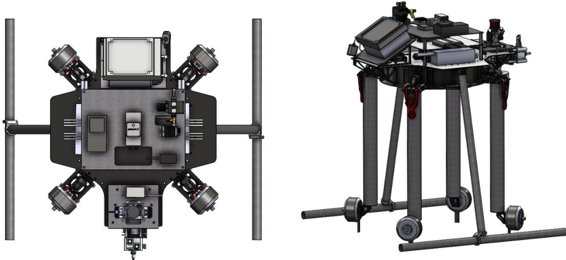
Figure 2: Oxcart with arms stowed. The Oxcart is designed to be easily transportable in a wide range of vehicles. The Oxcart when stowed can fit in the front seat of a normal sized passenger car.
