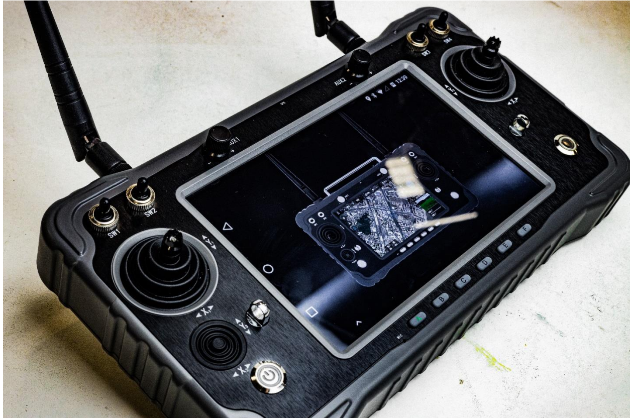
Figure 3: The handheld ground station controller for the Oxcart. This system provides the operator with multiple ways to interface to the vehicle. The operator can control the drone via the joysticks in manual and assisted modes, or the vehicle can operate fully autonomously via a waypoint mission uploaded from the controller. A real time HD video feed is present on the controller's screen. Multiple auxillary switches allow for controlling various payloads without the need for a separate controller or laptop computer.
